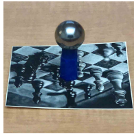
(a) A chrome ball placed on a marker serves as a GLEAM light probe.
