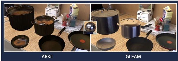
Figure 1: AR scene illuminated with ARKit (left) and GLEAM (right) illumination estimation, along with reflected environment in light probe (inset). GLEAM creates visual harmony between objects in virtual scenes and physical environments for improved photorealism.
