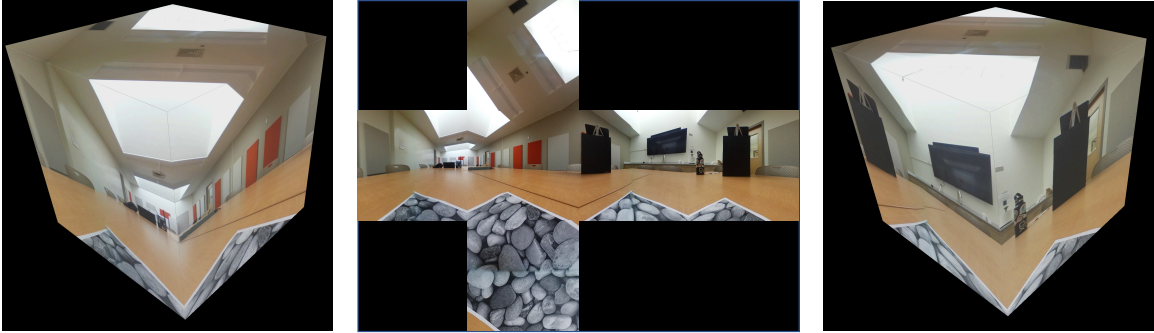
Figure 2.2: Cubemap representation (center) of environment maps. The figures on the left and right show the cubemap wrapped as a cube from two different viewpoints.
